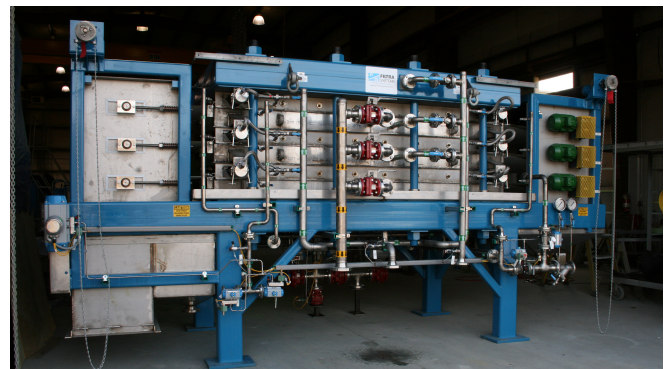
MINERAL CONCENTRATE DEWATERING This Verti-Press is designed to filter, cake wash and dewater an extremely valuable mineral concentrate. This 75 sqft machine produces cake that is up to 90% solids by weight.
