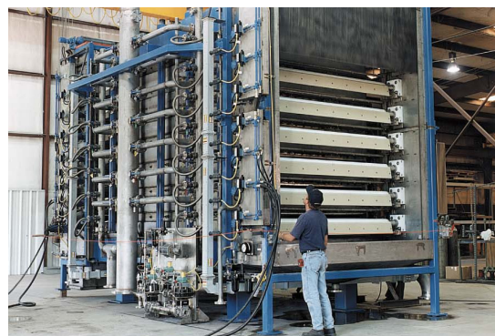
INDUSTRIAL MINERAL FILTRATION This 700 sqft filter is designed with 7 vertically stacked chambers and is expandable to 800 sqft. It is used to filter, pH adjust and provide an ion exchange cake wash in a single cycle.
