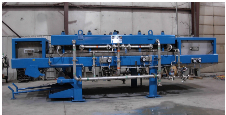
PROCESS WATER FILTER A 50 sqft Verti-Press. This filter is used by a fiberglass insulation producer to filter their process water. Fiberglass insulation, oils, greases, and resin is removed by using disposable media. The Verti-Press filter was chosen because it vastly improved filtration over conventional pressure filter technology.
